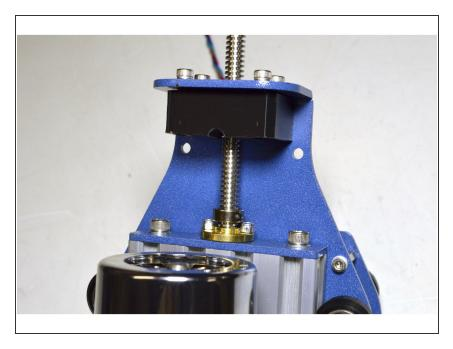
Insert the lead screw through the bearing block, through one 8mm Shaft Sleeve and screw it into the brass lead screw nut
