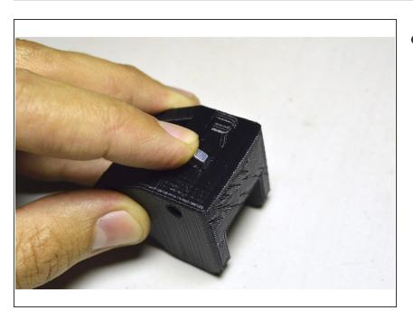
Slide the M4 Nuts (2 Pcs) into the slots provided in the Printed Parts
