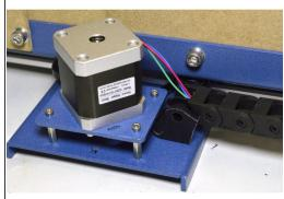
Click the Drag Chains into the printed brackets on both ends as shown
