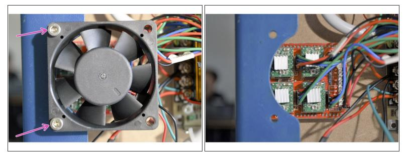
• Remove the two screws mounting the fan above the electronics
