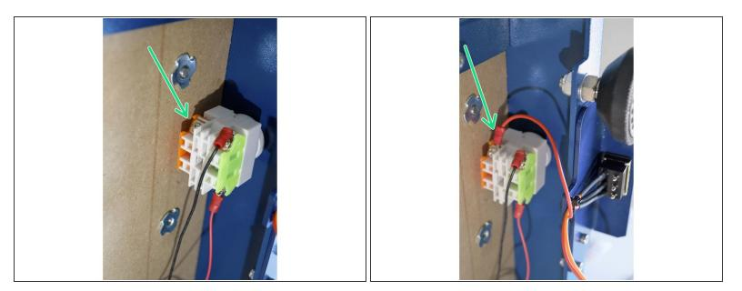
Connect the short red cable (centre pin on toggle switch) to the orange side (normally closed) on the E-Stop
