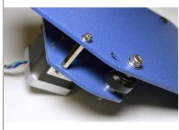
Fix the loose end of the M3x23 standoffs with the M3x8 cap screws (2 Pcs), M3 Washers (2 Pcs) and Pratley Pratlock
